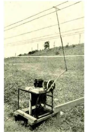
Copper wires separated by an insulating spreader being swung in a tie test to simulate the action of the wind. 1940
