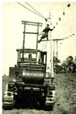
Brick hung on open wires to simulate ice load in line wire tie tests
