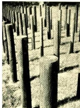
Life tests of telephone poles. 1940
