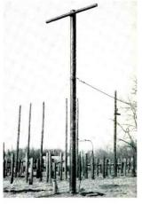
Fiberglas telephone poles are being tested for possible use. 1956
