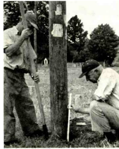
Wayne Parks and Bill check one of the poles in wood preservation experiment.
