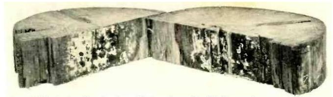
1932. Test section showing white fungal growth within the wood.
