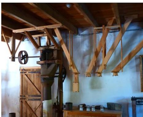
The bolter sifts the milled grain into different chutes by size from super fine to bran.
