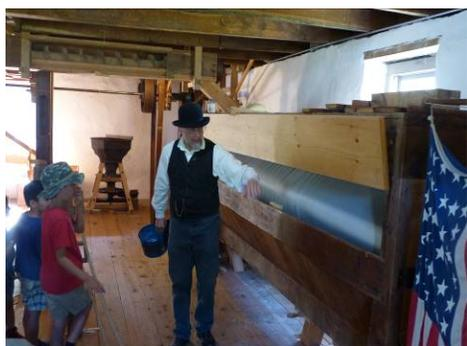
Ivins explains how the bolter separates the milled grain
